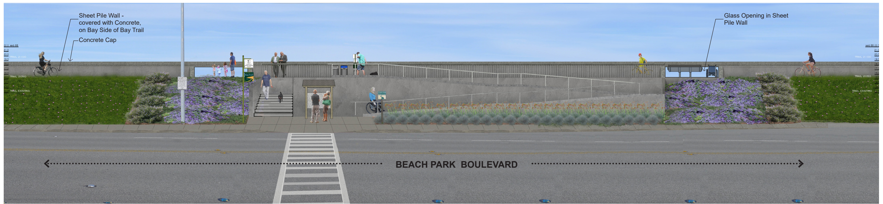
Typical View of Access along Beachpark Boulevard Levee Wall - Concrete Wall with Concrete Cap and 10'-0" Wide Glass Openings at Access Points
